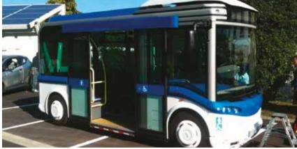
capture energy throughout the day and the then transfers it to a kind of transformer which is used to recharge the buses (the same way one would recharge a cellular phone using an electrical outlet) each evening (after the shuttle ends service) for eight hours.
